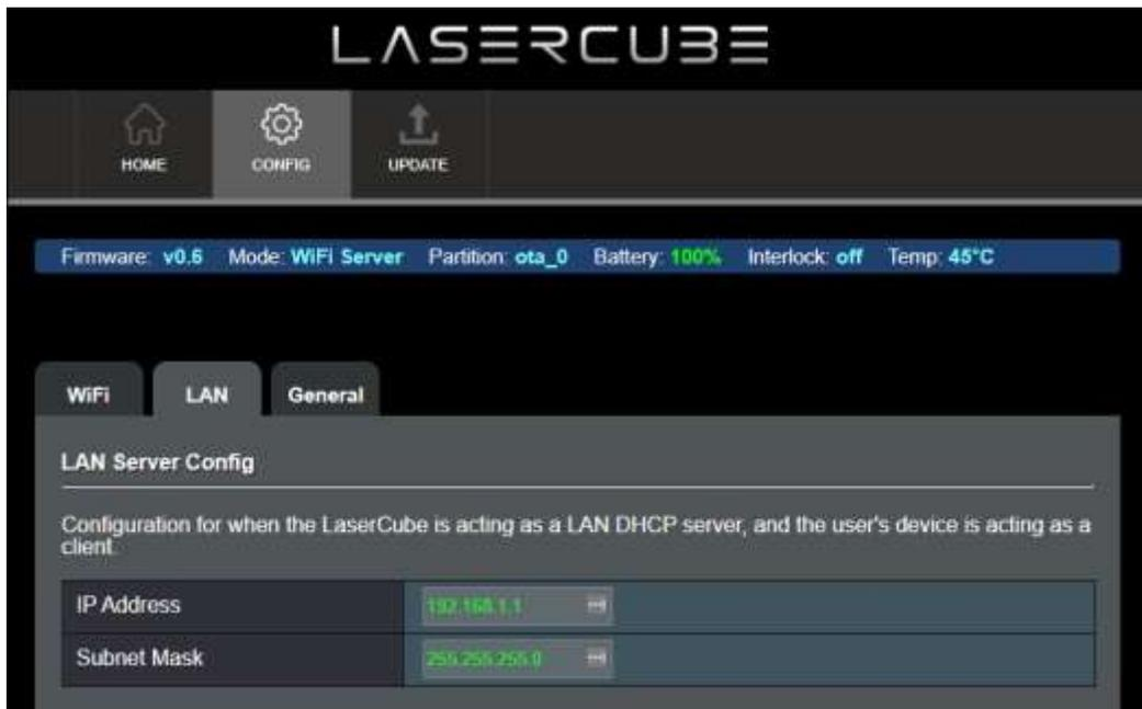
The IP address and subnet can be set for when the LaserCube is operating in LAN Server mode, where it provides a DHCP service.
